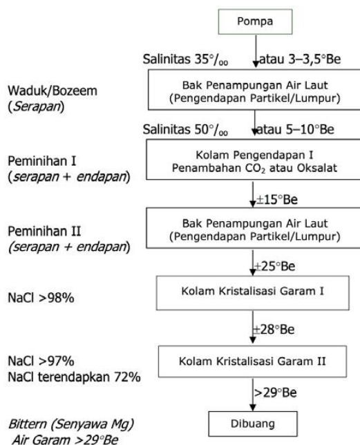
Gambar 12. Bagan proses pembuatan garam evaporasi kadar NaCl tinggi (Purbani, 2009)
