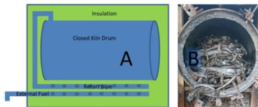
**Figure 1.** Schematic of closed drum retort kiln biochar production (A) and biochar produced with closed drum retort kiln (B)
