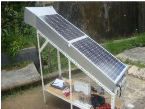
Fig 1 The experimental set up of PV/T system with air collector
