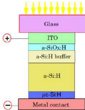
Fig.1 Sketch of proposed of the heterojunction solar cell structure Glass/ (ITO)/a-SiO x :H/(p)/a-Si:H(i)/n/a-Si:H(i)/μc-Si:H(n)/Ag.
