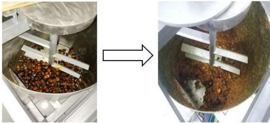
**Figure 3.** The test of FFB digester machine
