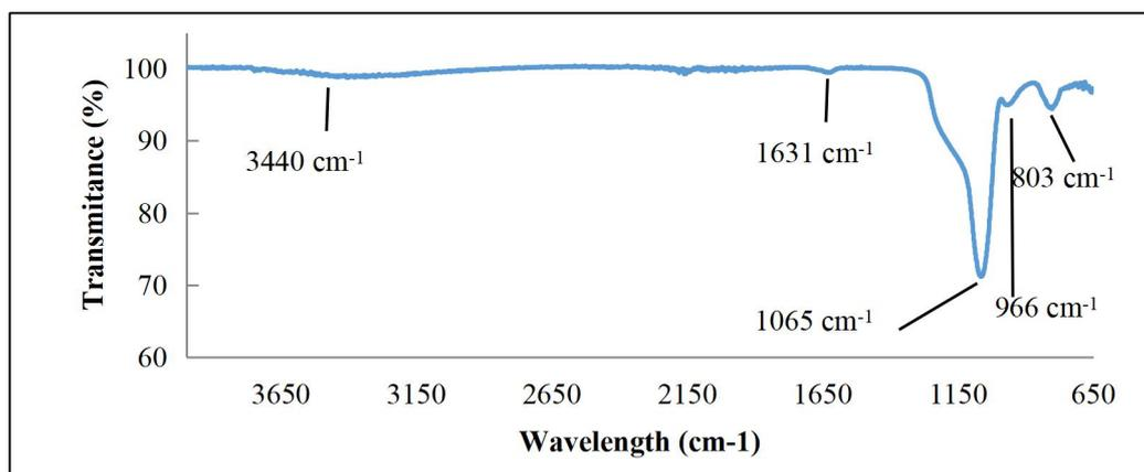
**Figure 3.** FTIR spectrum of SBA-15 material from rice husk ash
