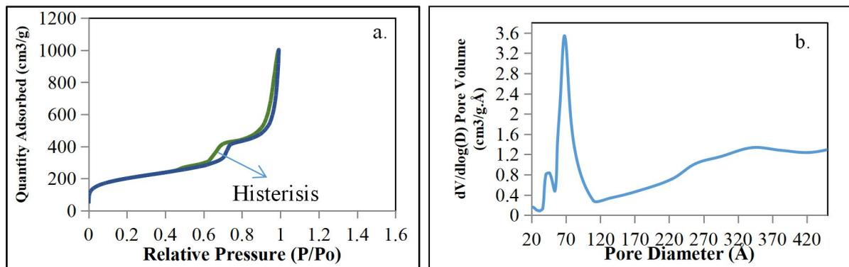
**Figure 1.** a. N<sub>2</sub> adsorption / desorption isotherm, b. Pore distribution of SBA-15 material from rice husk ash
