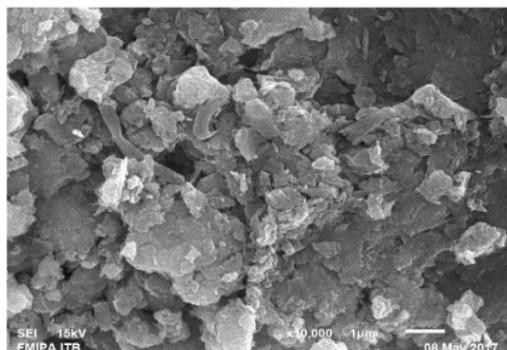
**Figure 3.** SEM image of DSBC-A 10.000 expand.
