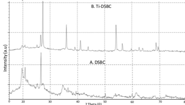
**Figure 2.** XRD results on (A) DSBC-A and (B) Ti-DSBC.
