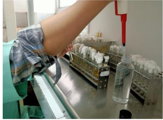
Gambar 8 Pipet air sampel
