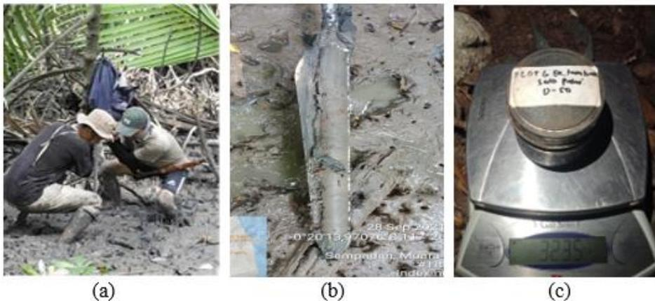
**Fig. 2.** Soil sampling: (a) soil sampling using peat drills (b) Soil samples on peat drill bits (c) soil samples are put in ring samples and weighed.
