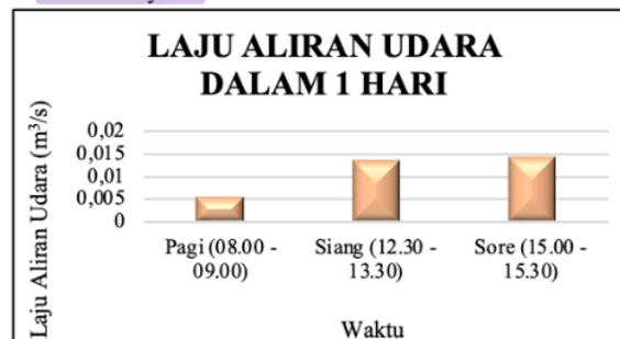
Figure 2. Airflow rate chart in 1 day in the tool room
