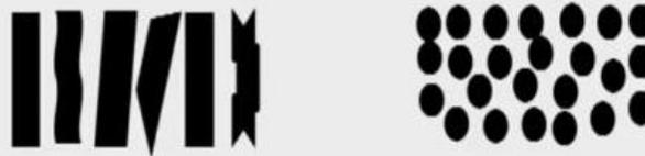
Figure. Some characteristic pore geometries found in porous membranes
