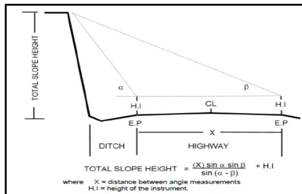
Fig. 5. Measurement of slope height. (Hock, E, Practical Rock Engineering, page 153)
