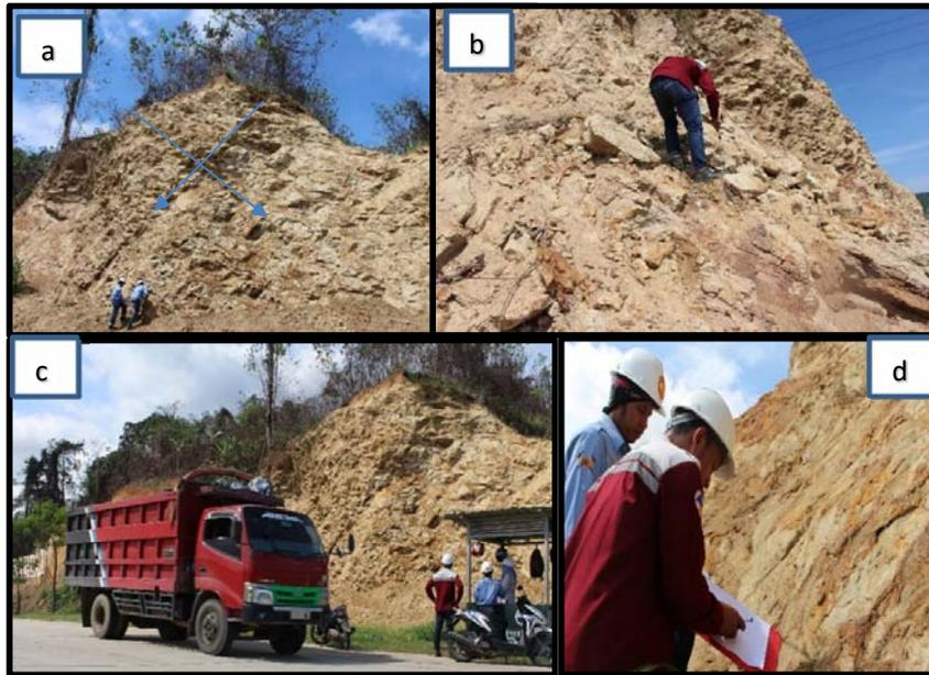
Fig. 7. (a) wedge failure, (b) slope condition, (c) vehicle risk, (d) discontinuities measurements
