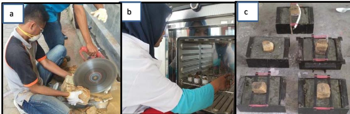
Fig. 8. (a) cutting process rock's block, (b) physical test process, (c) sandstone samples for slide test
