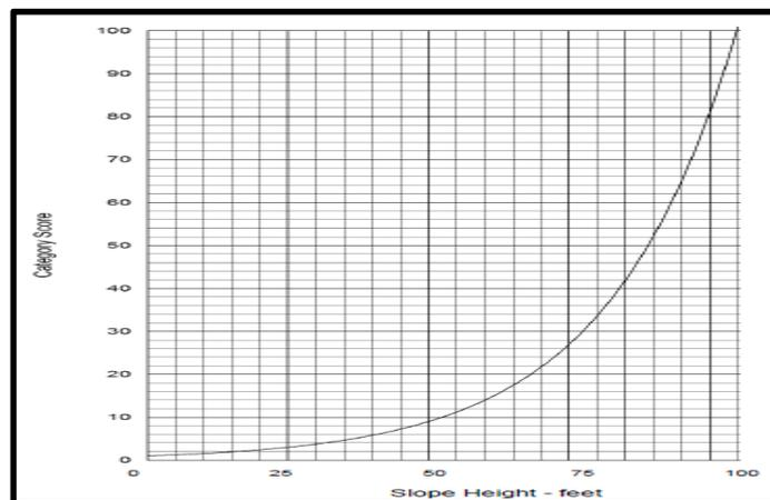
Fig. 3. Weighting graphic for slope height parameter (Hock, E, Practical Rock Engineering, page 151)
