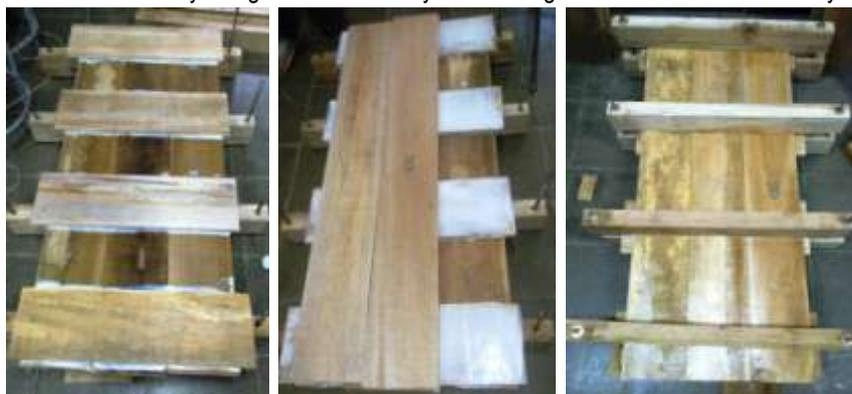
Figure 3. The construction of CLT floor.
