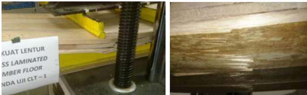
**Figure 8. Tension failure at the bottom of CLT floor**
