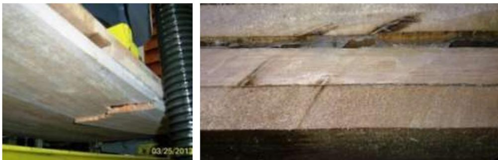
**Figure 9. Tension failure on the middle span of CLT floor (left) and failed in the PvAc glue (right).**
