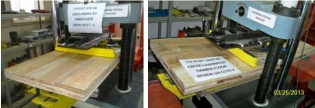
Figure 5. CLT floor under third point loading test
