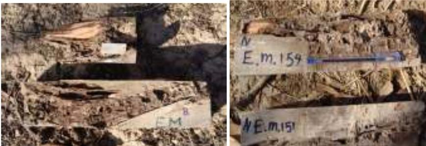
Fig 10-Control samples of *E. microtheca* in Albaji and Mishmast station, the attack by termites started after 36 month, then the grade No. reached to 0 and 2 after 96 month
