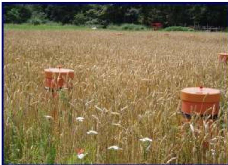
**Fig. 2: Closed chambers for gas sampling in a wheat field in Darmstadt, Germany in July 2007**
