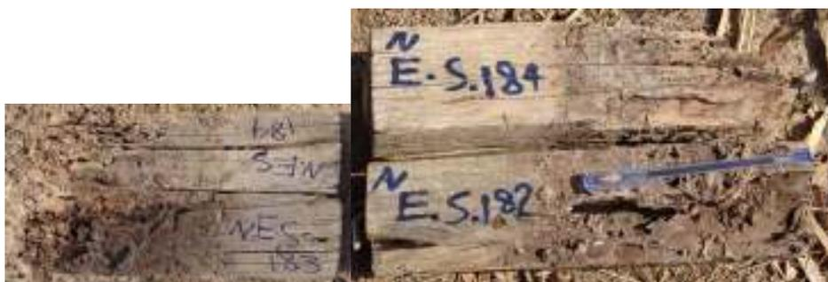
Fig 12- Control samples of *E. striatycalyx*, the attack by termites started after 24 month, then the grade No. reached to 2.4 after 118 month installation in Albaji and Mishmast station
