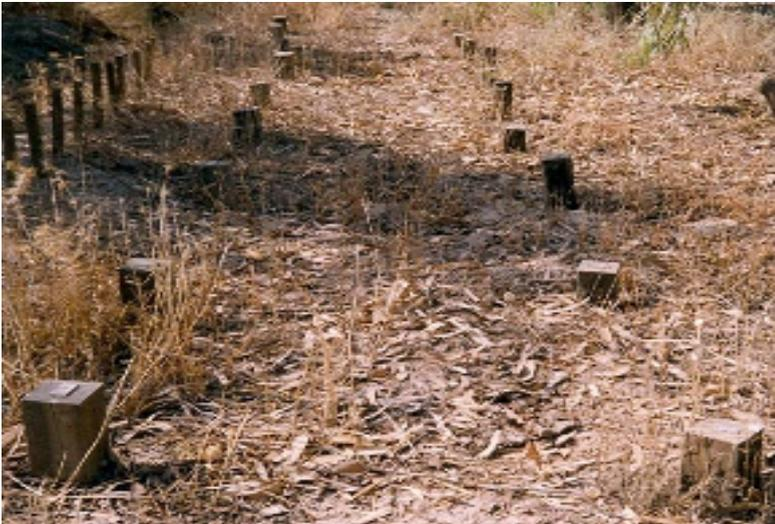
Fig 7- Samples impregnated with Creosote were sound after about 95 months
