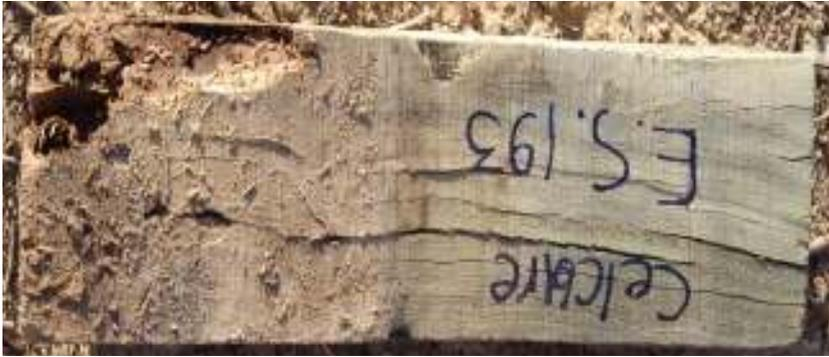
Fig 13- Treated with Celcure samples of *E. striatycalyx*, the attack by termites started after 36 month, then the grade No. Reached to 3 after 96 month installation in Albaji
