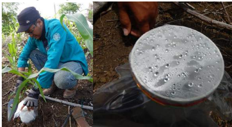
Gambar 4.12. Ilustrasi Cara Penanaman Soil Gas Chamber
