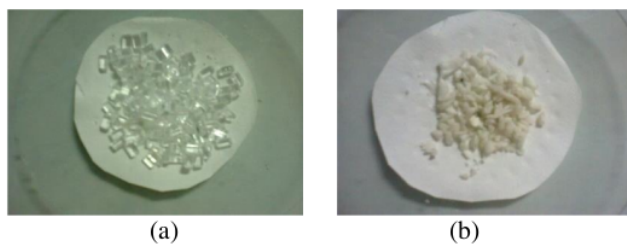
Figure 1. (a) Polystyrene resin before synthesis. (b) The synthesis result of MAP resin
