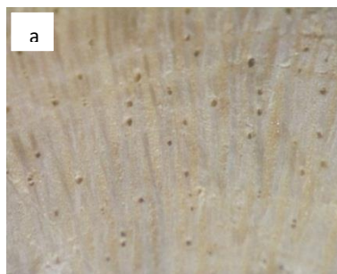
Figure 2. General view of transverse section: a. Vessel with diffuse porosity and radial arrangement. b. Rays. c. Fibers.
