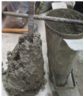
Figure 4. Preparation of B0 concrete for the slump test.
