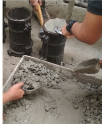
Figure 3. Preparation of concrete cylinder specimen.
