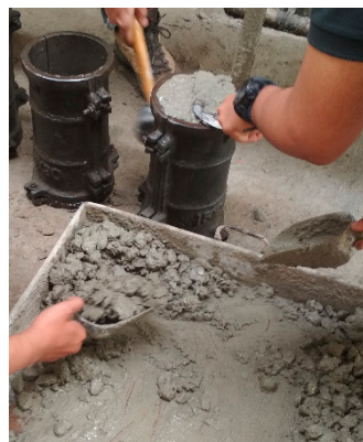
Figure 3. Preparation of concrete cylinder specimen.
