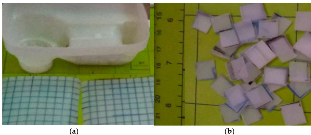
Figure 2. The preparation of high-density polyethylene (HDPE) addition: (a) marking procedure for the cutting process; (b) examples of HDPE lamellar particles with a size of 10 × 10 mm.
