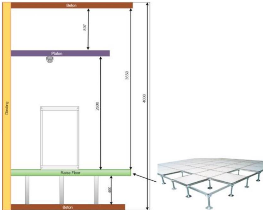
Gambar 40. Layout Raised Access Floor
