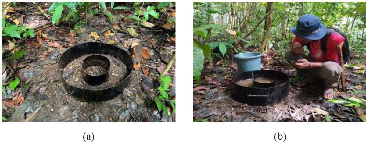
Figure 3. Double Ring Infiltrometer Installation to measure the rate of soil water infiltration (a), and to collect data on infiltration rate (b)
