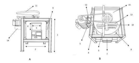
Figure 1. The design of palm fruit digester
