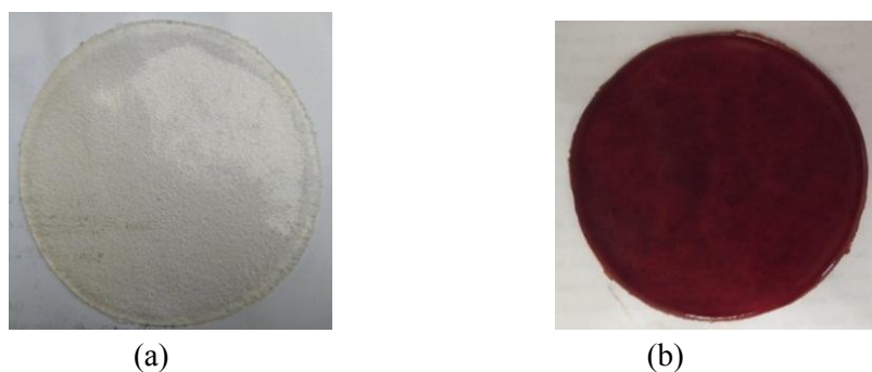
Gambar 2. (a) Edible Film Glukomanan Umbi Porang (b) Edible Film Glukomanan Umbi Porang + Ekstrak Etanol Umbi Bawang Tiwai
