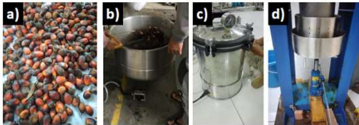
Figure 1. a) Oil palm loose fruits (LF), b) Steam pans, c) Autoclave, d) Mechanical press.
