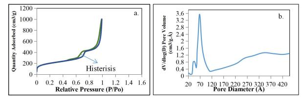
Figure 1. a. N<sub>2</sub> adsorption / desorption isotherm, b. Pore distribution of SBA-15 material from rice husk ash
