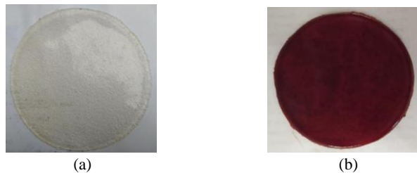
Gambar 2. (a) Edible Film Glukomanan Umbi Porang (b) Edible Film Glukomanan Umbi Porang + Ekstrak Etanol Umbi Bawang Tiwai
