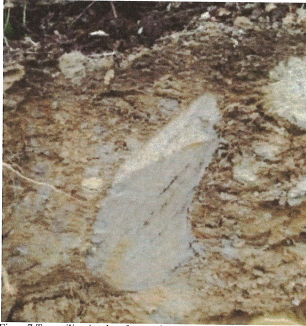
Figure7. Top soiling is taken from soft sandstone OB impermeable layers (Piece of sandstone , uncrushed, > 5 years)
