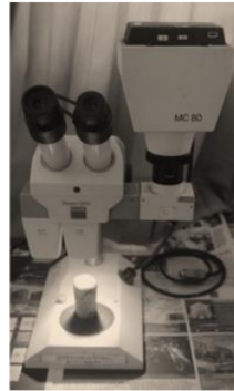
Figure 3 The process of observing the reaction wood using the Stereoscopic Microscope Nikon SMZ645 , after dripping with Zinc Chloride-iodine liquid
