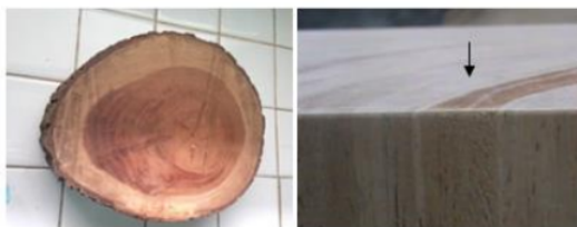
Fig 2. Wood Disk Sample Indicated as Reaction Zone
