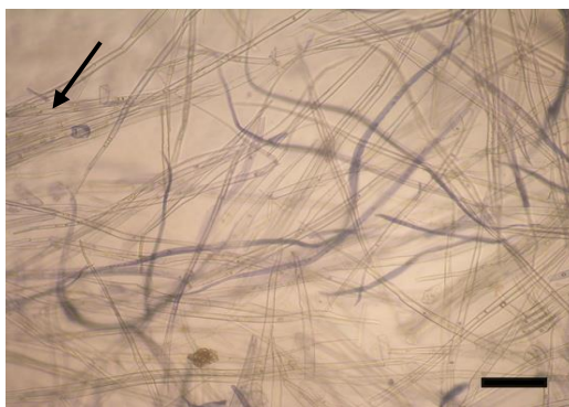
Fig 7. Reaction cell of Macerated fiber by Herzberg's Reagent
