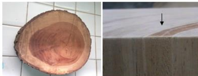
Fig 2. Wood Disk Sample Indicated as Reaction Zone
