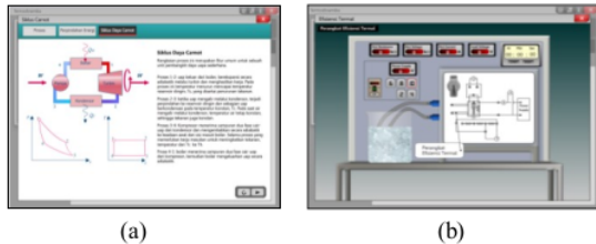
Figure 1. Examples of the Thermodynamics Interactive Multimedia presentations for the material of the second law of thermodynamics: (a) animation; (b) virtual experiment.
