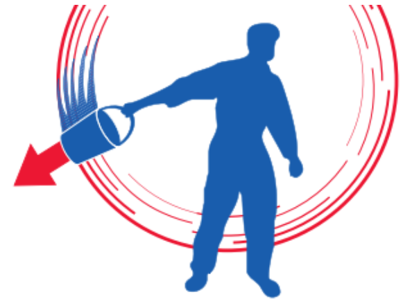
Fig. 6.2.13 Centrifugal force is generated in a rotating vessel .
