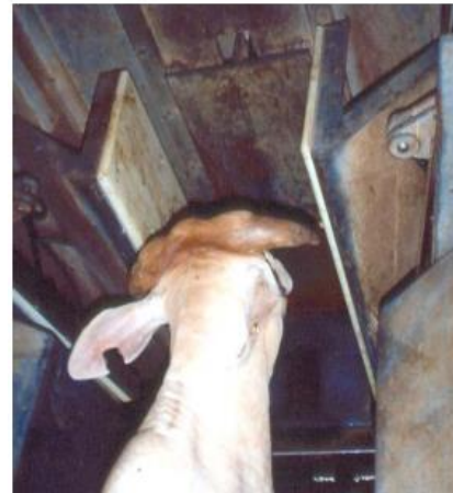
Fig. 70: Electrical stunning of cattle: The photo shows an animal about to enter a neck restrainer; once the animal is restrained, electrodes from a stunning device are placed on the nose and heart. This is an accepted Halal method used in a Jakarta abattoir.
