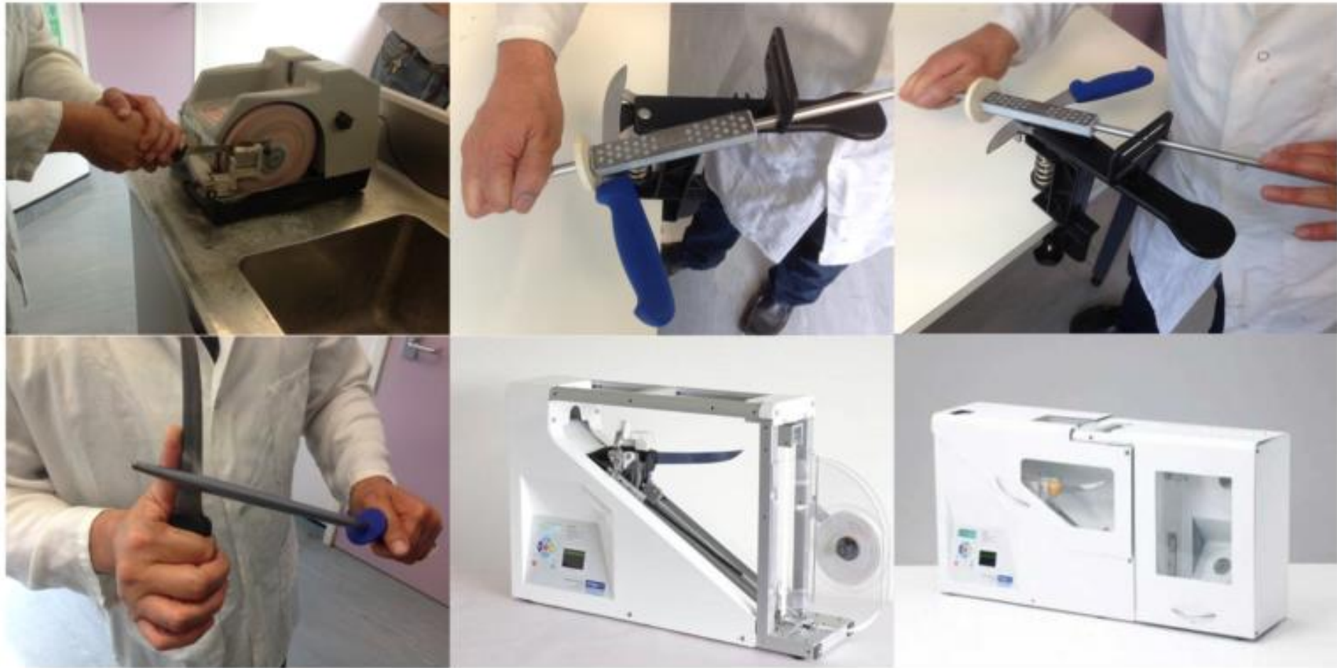
Fig. 3. Top to bottom, left to right: Photographs of steps involved in sharpening a knife from coarse grinding to steeling, and two versions of Anago Ltd. devices for quantitatively testing knife sharpness.
