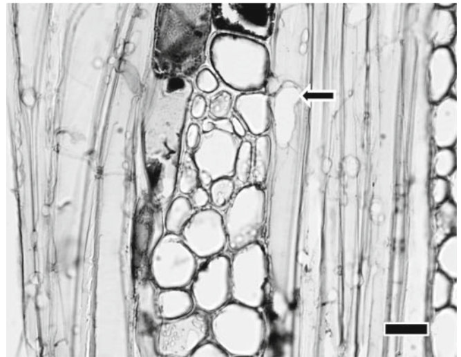
Fig. 5. Erosion channels with U-notches in fiber cell wall (arrow). The sample was prepared from site A shown in Fig 1b. Bar 20 \mu\text{m}
