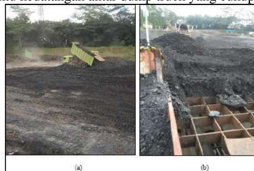
Gambar 15. Kegiatan (a) Dumping, (b) Trimming ke Hopper
