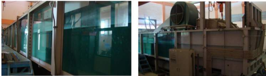
Figure 3 (a) Flume tank; (b) wave generator
