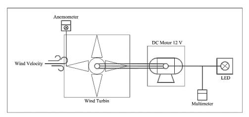
Figure 2. PLTB prototype system testing configuration
