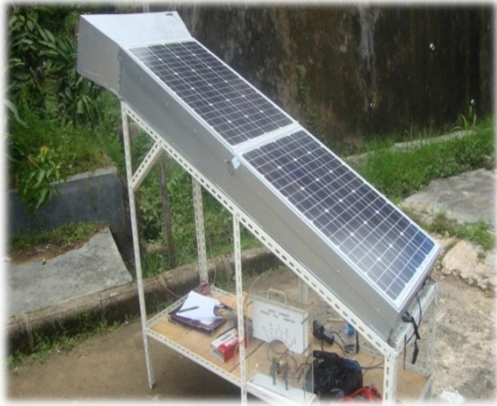
Fig 1 The experimental set up of PV/T system with air collector
