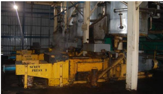
Gambar 6.9 : Mesin screw press terintegrasi mesin digester
