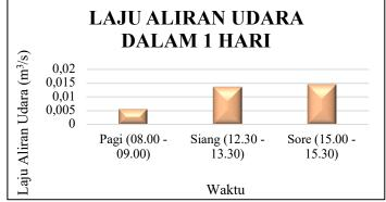
Figure 2. Airflow rate chart in 1 day in the tool room
