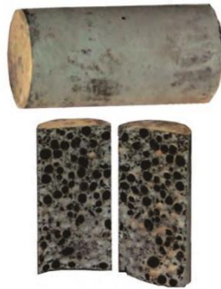
Gambar 2.3. Beton Ringan Lusi (Dinas PUPR Kulun Progo, 2020)
