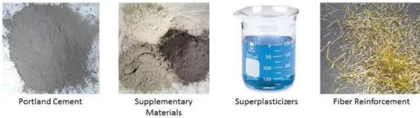
Gambar 5.3. Proporsi Campuran Ultra High Performance Concrete (UHPC) ( “Ultra-high-Performance Concrete: Characteristics, and Applications - the Constructor,” 2019)
