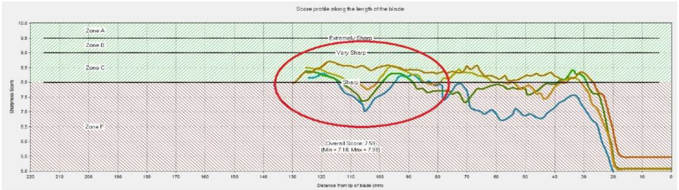
Figure 8 - Stone sharpened tests show a drop of 1.5 in the sharpness score after 90 cuts
