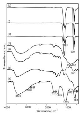
**Figure 1.** FTIR spectra of (a) CFB, (b) CuO, (c) Fe<sub>2</sub>O<sub>3</sub>, (d) TiO<sub>2</sub>, (e) Fe<sub>2</sub>O<sub>3</sub>/CFB, (f) CuO/CFB and (g) TiO<sub>2</sub>/CFB.
