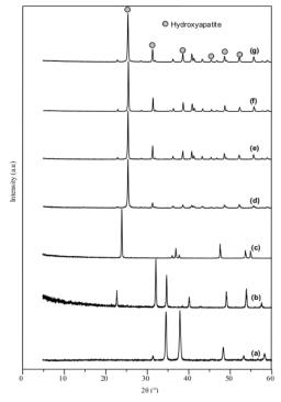
**Figure 2.** XRD pattern of (a) CuO, (b) Fe<sub>2</sub>O<sub>3</sub>, (c) TiO<sub>2</sub>, (d) CFB, (e) Fe<sub>2</sub>O<sub>3</sub>/CFB, (f) CuO/CFB and (g) TiO<sub>2</sub>/CFB.
