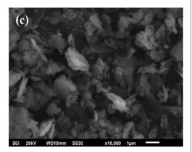
Figure 3. SEM images of (a) Fe<sub>2</sub>O<sub>3</sub>/CFB, (b) CuO/CFB and (c) TiO<sub>2</sub>/CFB.
