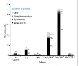
Figure 5. Comparison of catalytic Fromance of no catalyst, TiO<sub>2</sub>, CFB, Fe<sub>2</sub>O<sub>3</sub>/CFB, TiO<sub>2</sub>/CFB and CuO/CFB catalysts in the oxidation of styrene (5 mmol), 30% H<sub>2</sub>O<sub>2</sub> (5 mmol) and catalyst (50 mg) at room temperature for 24 h.
