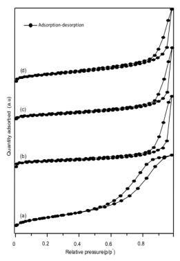
**Figure 4.** The physisorption isotherms of (a) CFB, (b) Fe<sub>2</sub>O<sub>3</sub>/CFB, (c) CuO/CFB and (d) TiO<sub>2</sub>/CFB.
