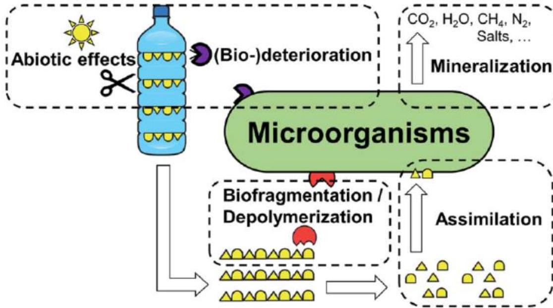
Schematic illustration of plastic biodegradation (Lucas *et al.*, 2008).
