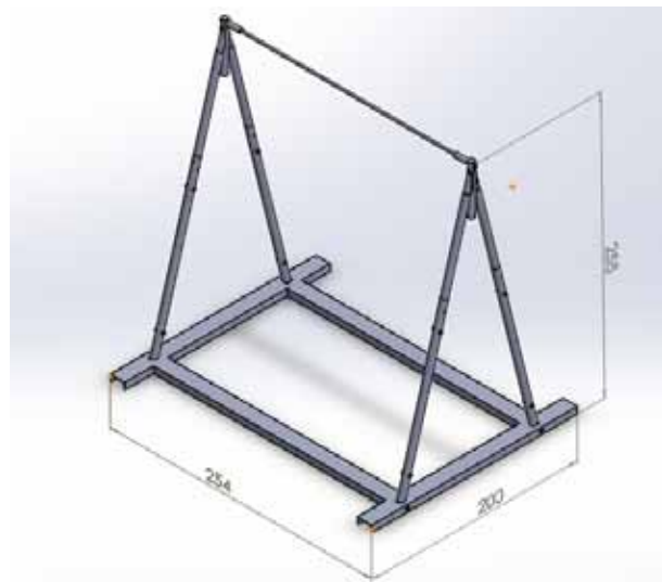
Figure 4. Design of the single crossbar tool
