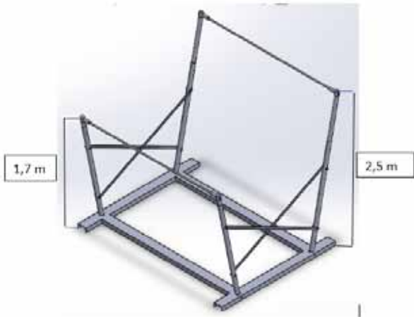
Figure 3. The design of the multilevel crossbeam tool
