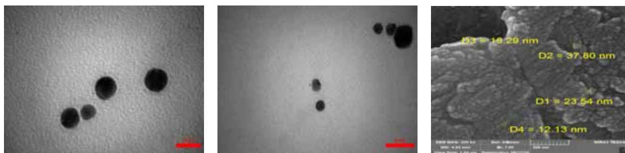
Figure (3)a: FE-SEM images recorded by deposited gold-DW nanoparticles on pure glass slide; b,c: TEM image of gold nanoparticles prepared by Biological method using Bacteria supernatant
