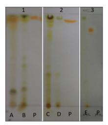
Fig. 2: Identification alkaloid using Dragendorff spray reagent,
