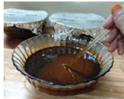
FIGURE 1. Delignification process on wood powder when soaking with 5% NaOH for 2 hours.
