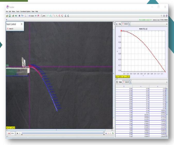
Fig. 2. Procedure for estimating the elastic modulus of the beam
