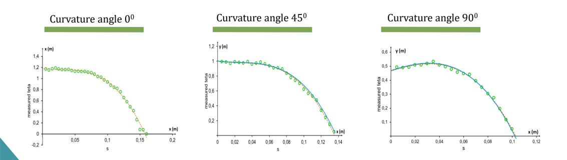
Fig.5 Experimental data fitting graph (green colored round shape), theory (orange dashed line) and simulation (blue line) on rectangular sample for Curvature angles 0<sup>0</sup>, 45<sup>0</sup> and 90<sup>0</sup>
