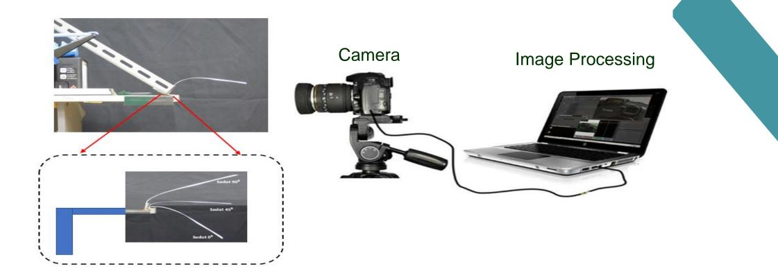
Fig.1. Illustration of a Simple Experiment Measurement Elasticity Modulus for Copy Paper 100gsm
