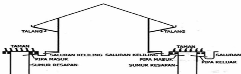
Gambar 4.1.: Sumur Resapan Kosong(Sharuel 2010)
