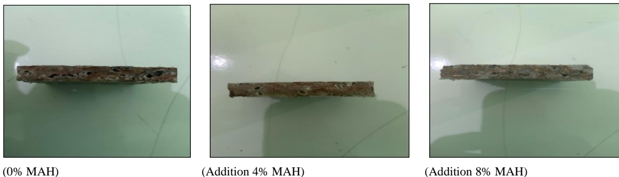
Figure 10. The Number and Size of Cavities in WPC Decreased with the Addition of MAH.
